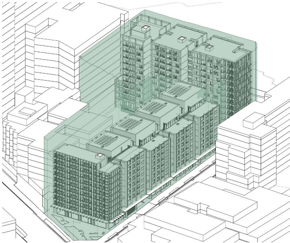
Figure 36: Height of Building encroachments
